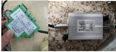
Figure 8. Signal amplifier and signal converter.
