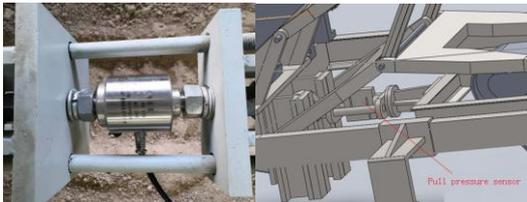
**Figure 3.** Follow-up lifting tension and pressure testing device.
