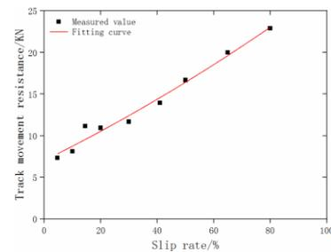
Figure 12. Curve of motion resistance changing with slip rate.
