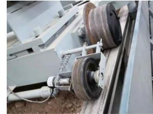
**Figure 5.** Trolley angle encoder.
