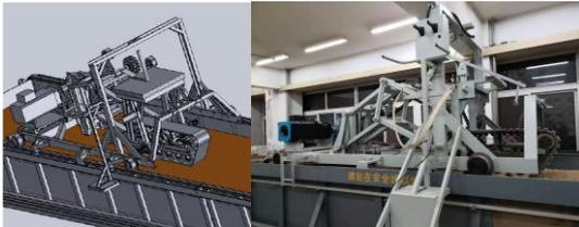
**Figure 2.** Design drawing and physical drawing of soil tank and test trolley.
