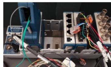
**Figure 7.** Chassis and acquisition module.
