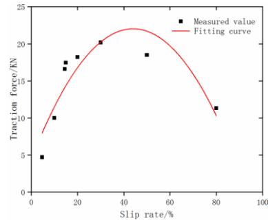
Figure 11. Curve of hook traction force changing with slip rate.
