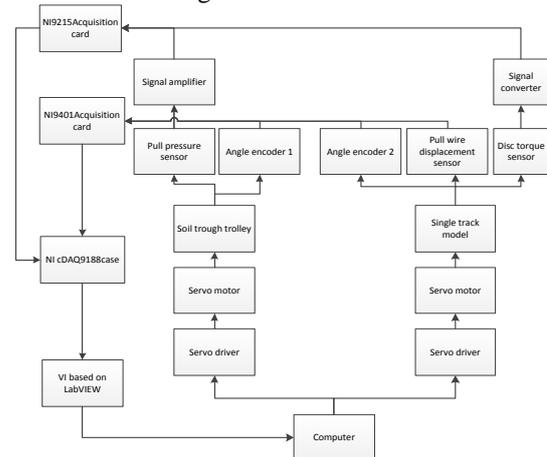
**Figure 1.** Schematic diagram of sensor and test acquisition system of soil tank test bench.
