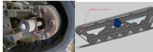
**Figure 6.** Physical drawing and installation position of track model angle encoder.
